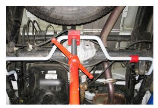
29. Carefully bend the hydraulic line away from the axle and place the U-bolts inside the lower shock mount brackets, over the axle tube, and under the brake line. Ensure the brake line is not clamped underneath. Place the U-clamp on the U-bolt followed by the support plate. Mount the sway bar and bushing bracket on the U-clamp. Hand tighten the supplied nuts on the U-bolt for now. Ensure the sway bar is positioned below the axle.
