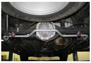
32. Torque the lower end link bolts to 40 ft lbs.
