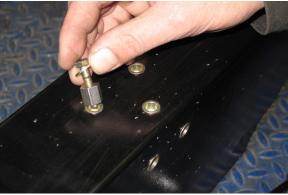
19. Using a 1/2" wrench on the hex tool and a 7/16" wrench on the bolt, tighten the bolt to lock each nut insert into the frame.
