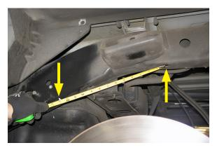
11. Use a marking pen to mark the edges of the bracket onto the frame as shown.
