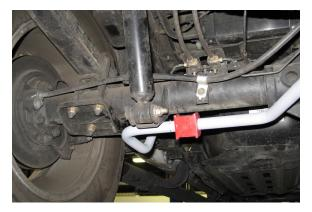
27. Ensure there is 1/32" to 1/16" of the bushing is showing after the bracket is seated. If the bushing is showing more than 1/16", use a sander or a sheet of coarse grit sandpaper to shave it down to the proper height.
