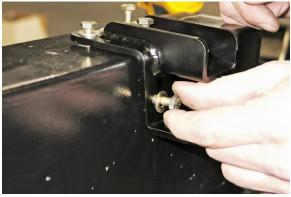
22. Attach the end links to the end link brackets with two 3/8-16" x 2-1/2" bolts, four washers, and two 3/8" stover lock nuts. Torque the upper and lower end link bolts to 40 ft lbs.
