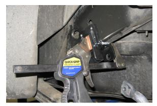
13. Detach the clamp and remove the end link bracket from the frame.
